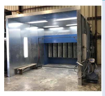
**Automated Filter Maintenance:** Adjustable time based, reverse-pulsing of filters for longer life and optimum booth air flow. Showerhead valve provides superior cartridge cleaning
