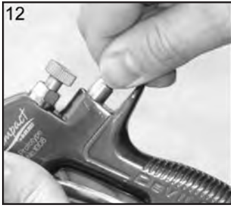
12. Fit Valve Seat to Gunbody.
