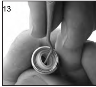
13. Remove Rear Air Valve Seal from housing (10) with a hooked instrument.
