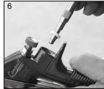
6. Remove Valve Seat.
