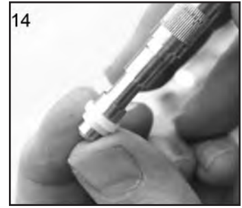
14. Fit new Seal to Service Tool.
