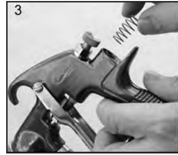
3. Remove Housing (10) and Air Valve Spring.
