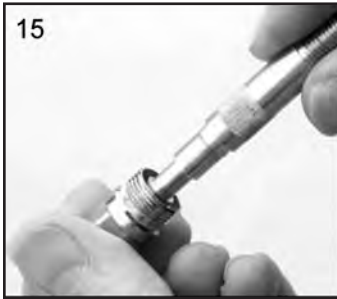
15. Fit Seal to Housing (10).
