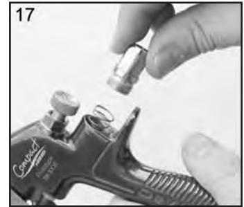
17. Replace Valve Spring and screw in Housing (10).
