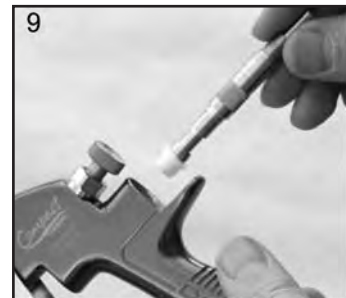
9. Fit New Front Seal to Service Tool.
