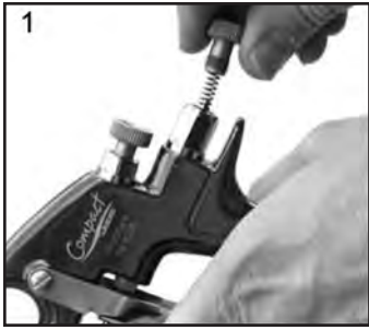
1. Remove Adjusting Knob (7), Spring (8), and Needle (9).
