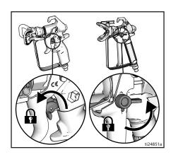
Turn ON/OFF switch to OFF position. Wait 7 seconds for power to dissipate.
