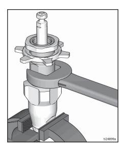
Install o-ring onto packing nut. Torque to 75 ± 5 ft-lb (101.7 ± 6.8 N•m) or additional 1/2 turn from hand tight.
