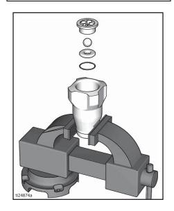
4. Tap piston rod out of cylinder with a hammer or flip over and tap piston rod out against a bench.
