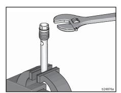
6. Clean and inspect parts. (The piston has a special thread locking/sealing patch. Apply thread sealant to the threads.
