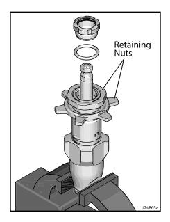
2. Unscrew cylinder from intake valve.
