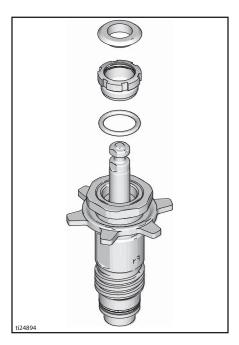
6. Apply liberal amounts of grease or oil to piston packings.
