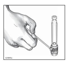
Grease top inch or two of piston rod that will go through the cylinder throat packings. Gently guide displacement rod up through throat packings. Tap bottom of piston valve as necessary with a leather or plastic hammer.
