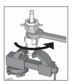
Dissemble intake valve. Clean and inspect. O-ring may require a pick for removal.
