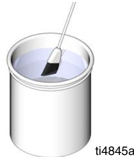
FIG. 14: Use solvent-dipped soft-bristle brush
