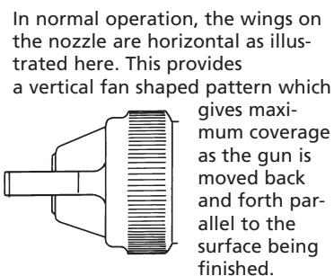
In normal operation, the wings on the nozzle are horizontal as illustrated here. This provides a vertical fan shaped pattern which gives maximum coverage as the gun is moved back and forth parallel to the surface being finished.
