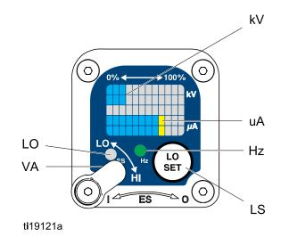
Figure 2 Smart Gun Module in Operating Mode
