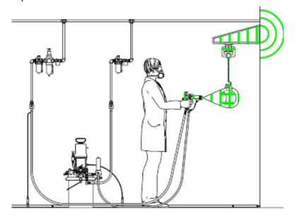
Figure 13 Ground the Object Being Sprayed
