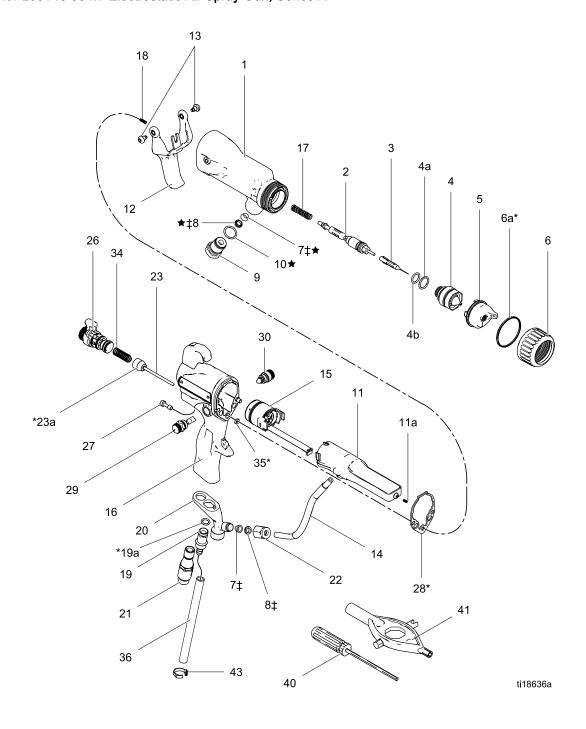
Part No. L40T10 40 kV Electrostatic Air Spray Gun, Series A
