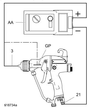
Figure 17 Test Gun Resistance
