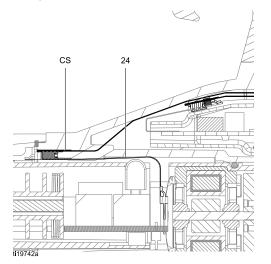
Figure 27 Connect Flexible Circuit
