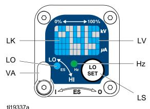
Figure 5 Low Voltage Setting Screen (Locked)
