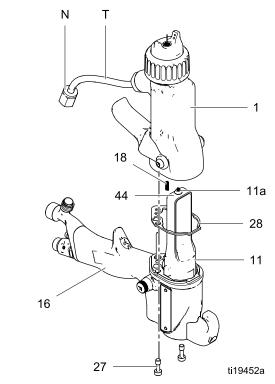
Figure 25 Barrel Installation
