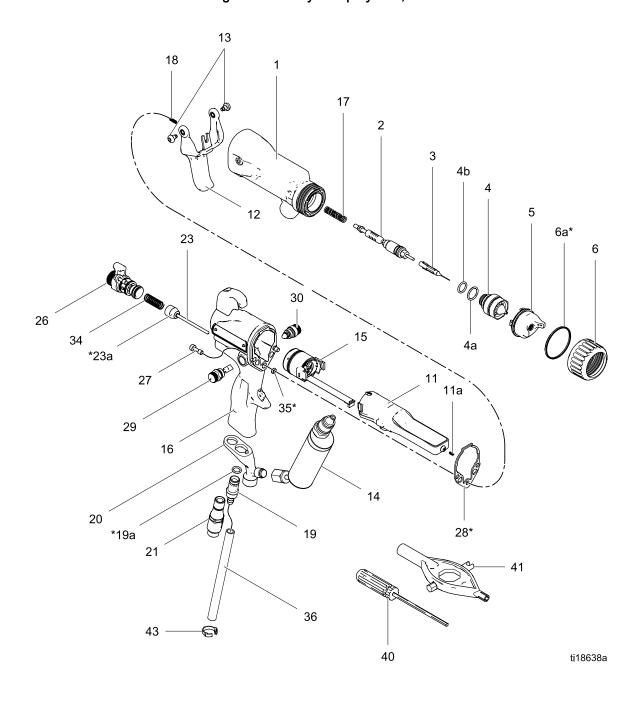
Part No. L40T16 40 kV Electrostatic High Conductivity Air Spray Gun, Series A Part No. L40T15 40 kV High Efficiency Electrostatic Air Spray Gun, Series A Part No. L60T16 60 kV Electrostatic High Conductivity Air Spray Gun, Series A Part No. L85T16 85 kV Electrostatic High Conductivity Air Spray Gun, Series A
