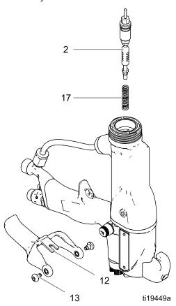
Figure 22 Fluid Packing Rod Removal
