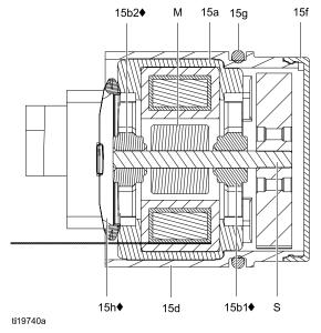
Figure 29 Alternator Cross-Section
