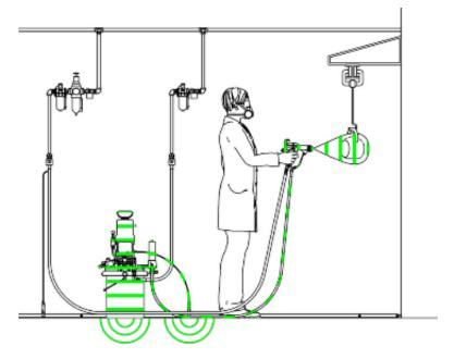
Figure 15 Ground the Fluid Supply
