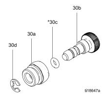
Figure 32 Fan Air Adjustment Valve
