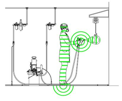
Figure 12 Ground the Operator
