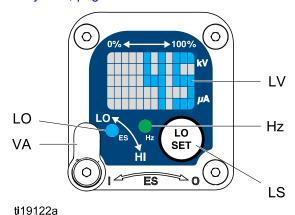
Figure 4 Low Voltage Setting Screen (Unlocked)
