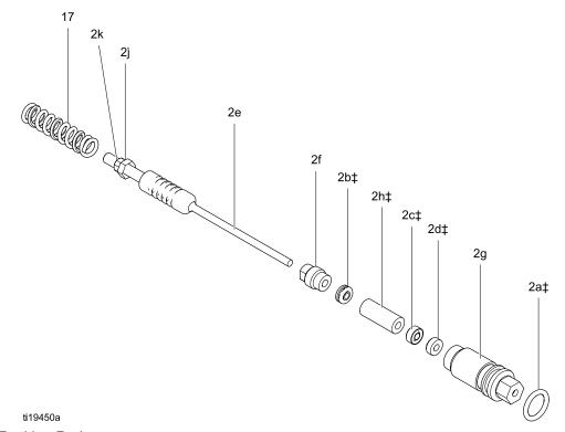
Figure 23 Packing Rod
