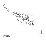
Electrostatic Air Spray Gun: ground the gun by connecting the Graco Grounded Air Hose (AH) to the gun, and connecting the air hose ground wire to a true earth ground. See Check Gun Electrical Grounding, page 25.
