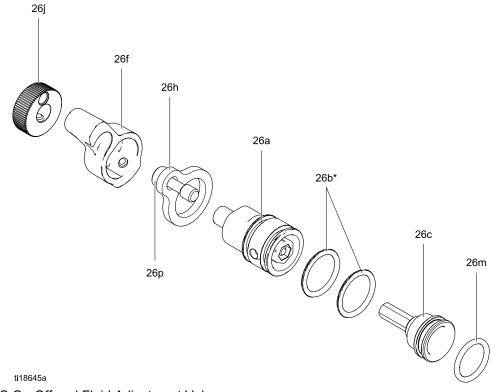
Figure 34 ES On-Off and Fluid Adjustment Valve
