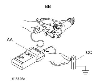
Figure 16 Check Gun Electrical Grounding
