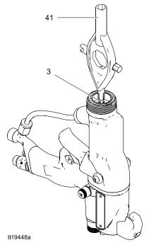
Figure 21 Electrode Replacement
