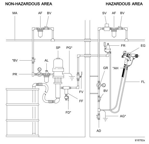
Figure 10 Typical Installation
