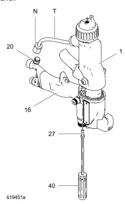
Figure 24 Barrel Removal
