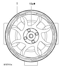
Figure 28 Fan Orientation
