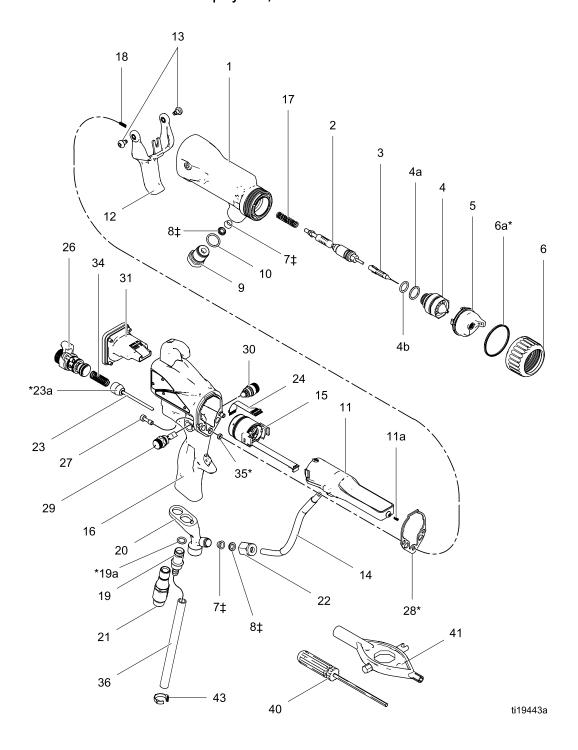
Part No. L60M10 60 kV Electrostatic Air Spray Gun, Series A
