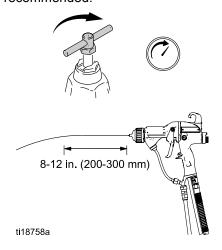
21. Turn on the air to the gun. Turn ON (I) the ES On-Off switch (J).
