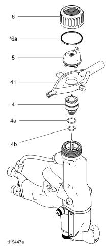
Figure 20 Air Cap and Nozzle Replacement
