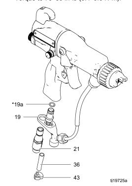
Figure 37 Air Inlet Fitting and Air Exhaust Valve
