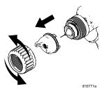
6. Clean the air cap, retaining ring, and nozzle with a soft brush and compatible solvent.
