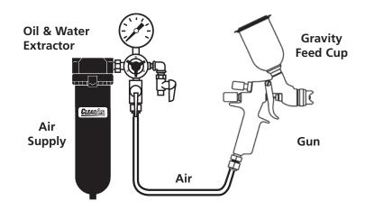
Air pressure for atomization is regulated at the extractor. The flow of the fluid is adjusted by the fluid valve control knob on gun, viscosity of paint and air pressure.
