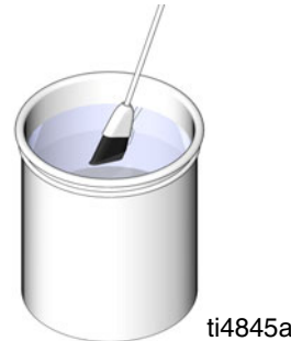
FIG. 15: Use solvent-dipped soft-bristle brush
